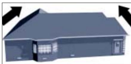
If you are building a new home, the type and shape of the roof can help determine how well it will perform during a severe windstorm. A **hipped roof** typically performs better in windstorms than a gabled roof because of its aerodynamic properties. A hipped roof slopes upward from all sides of the building. A **gabled roof** has two slopes that come together to form a ridge or peak at the top, making each end look like the letter A.
