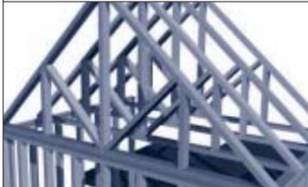
Brace the intersection of the gable and the end wall. This intersection is a particularly weak point and those that are not properly braced can collapse, causing major damage. In homes with attics, an attic floor or ceiling diaphragm with the proper bracing techniques can be used to provide the lateral support of the gable end wall if the end wall is NOT framed full height, or ballooned framed.
