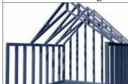
Homes with high, cathedral ceilings, where there is no place to brace a gabled end should be **balloon framed**. Use full-height studs, concrete or solid masonry walls from the floor below all
